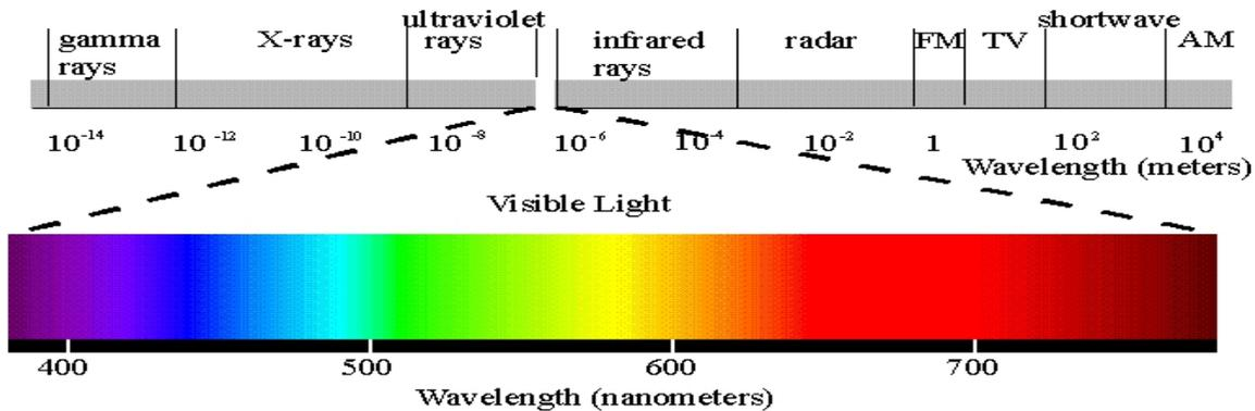
The electromagnetic spectrum with the visible light section enlarged to show visible light.
