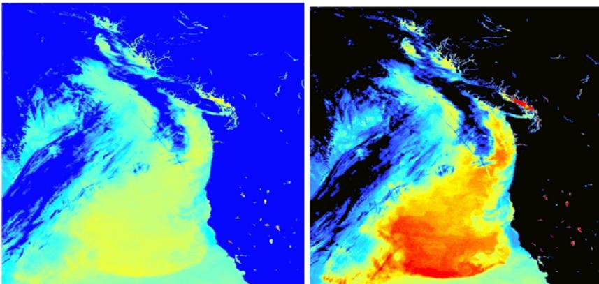
The image on the left has not been stretched and because most of the variation in temperature is in a small range it does not show up well. In the right image, the color range has been stretched over a smaller range of values where most of the data in this image occurs.
