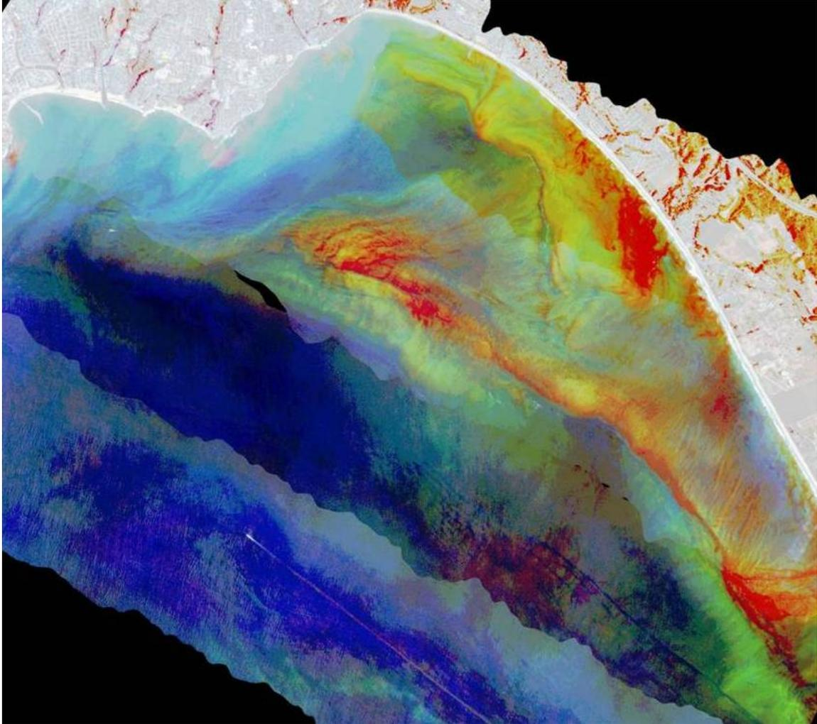
**Figure 2.** SAMSON image of the northeast corner of Monterey Bay. This is the third map collected on September 12, 2006. The bloom is identified using the 709 nm band and is indicated in red in the image. The adjacent regions in yellow also have high levels of phytoplankton. The bloom is a mix of species, but predominately the dinoflagellate *Akashiwo sanguinea*. Four flight lines are shown that have been geolocated to one pixel accuracy and mosaiced to produce the image.
