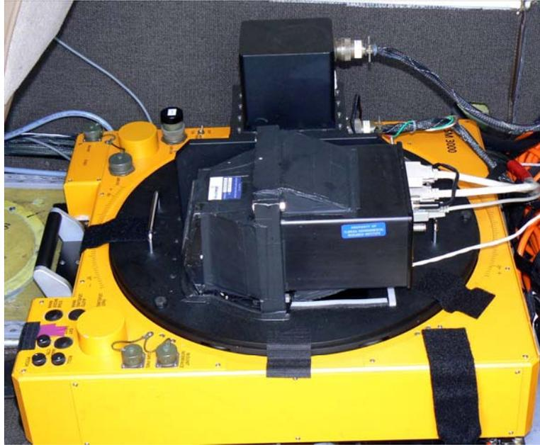
**Figure 1.** The Spectroscopic Aerial Mapper with On-board Navigation (SAMSON). The hyperspectral imager is black object in the foreground. The black box at the top of the image is the integrated inertial navigation system which sits atop a high resolution framing camera. The yellow frame is the motion compensation mounting system.
